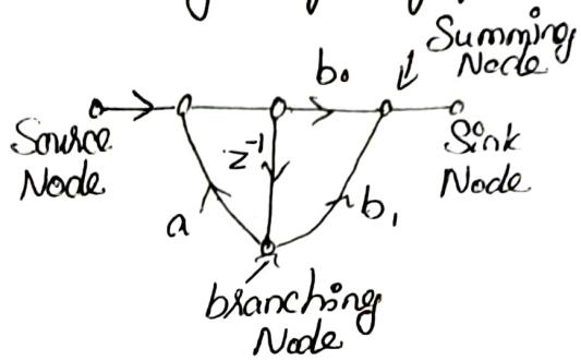
Signal flow graph contains the same basic information as the block diagram realization of the system. Only difference is that both branch point & adders in the block diagram are represented by nodes.
